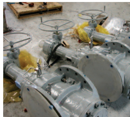
Array Accuseal (R) DB&B Expanding Plug Valve ready for packing and sending out
